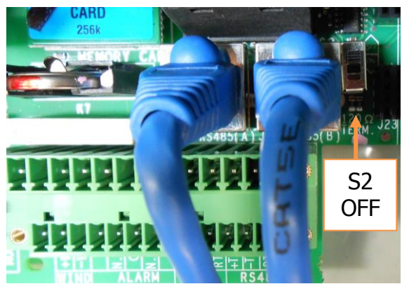
ABB loop-through: S2 OFF (Terminator OFF)
