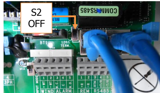
ABB loop-through: S2 OFF (Terminator OFF)
